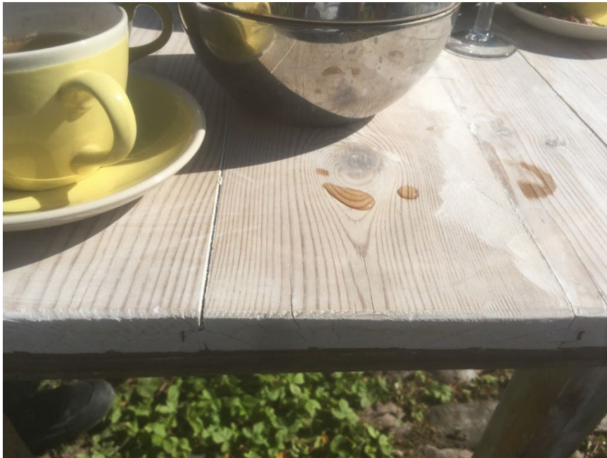
Wooden boards on a garden table, treated with lime soap treatment. Notice how water droplets bead off the surface - for some time before they soak in.
